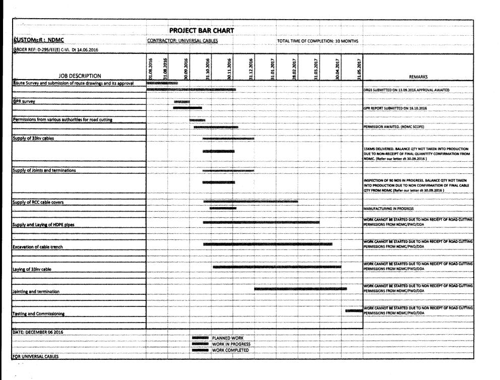
Project:-PCTABLISHING TWO 33 KV ESS AT KIDWAI NAGAR (EAST)
